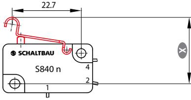
**!** *Note: To ensure the proper working of the positive opening operation it is necessary to depress the plunger to the point of total positive opening travel. However, it must not be pushed beyond total travel position. Data is valid for new switches.*
