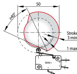
**Switch with roller lever actuated by linear cam**
