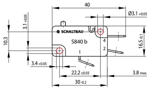
**Switch with roller lever actuated by cam disc**
